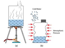
• When a can filled with hot water is closed and is cooled down rapidly by pouring cold water on it, it will crash instantly.
